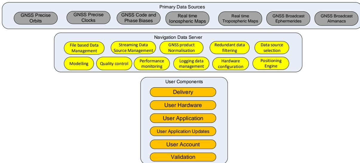
Figure 2 - DDK Service Components
