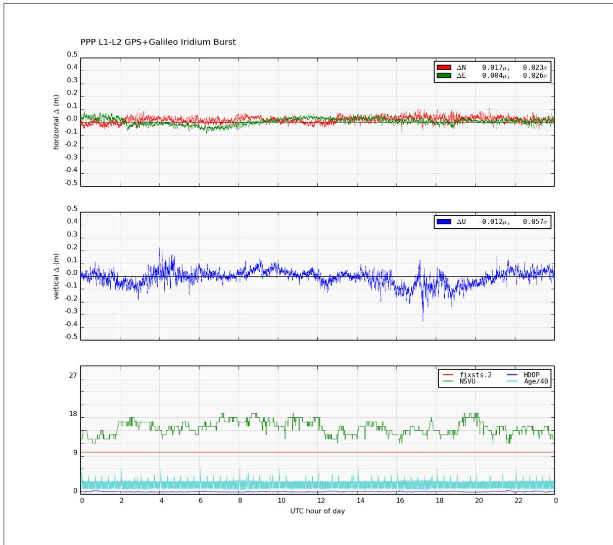
Figure 5 – Iridium Burst Delivery: Coordinate Position Δ Values
